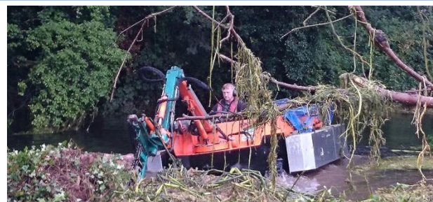
Photos Left: Removal using long reach excavator Right: Removal using truxor boat (source EA)
